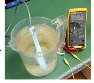
positioned diagonally in the container (about 17 cm, or 7" deep). The readings you obtain may differ from stated if you use a different container.
